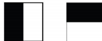
Fig. 5. The Haar wavelet filters used to describe the interest points.
